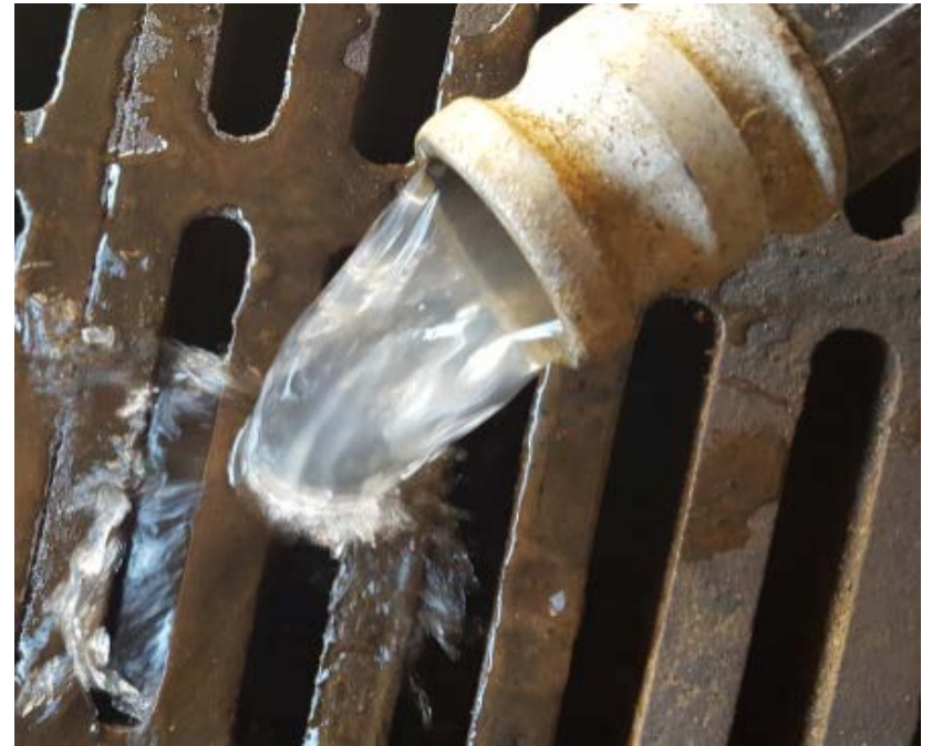
Pressate (Filtrate) During Dewatering
